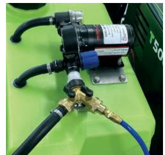
Brass, threaded, control valves to adjust flow rates or switch between wand and front spray nozzle.
