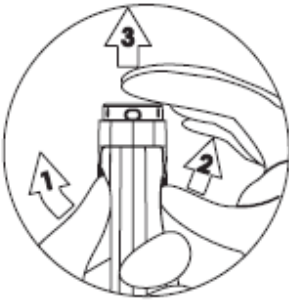
Fig. 1: Removing battery cover
